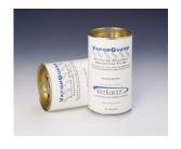
The **VetEquip®** VaporGuard Absorption charcoal filter (pictured to the left) does not require upright positioning. It ventilates only through the top and may be used properly whether on a solid surface or on its side. \*Replace this canister after a 50 g increase from initial weight recorded.
